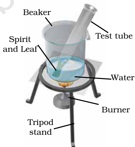
Figure 4.1 Set-up for extraction of chlorophyll
